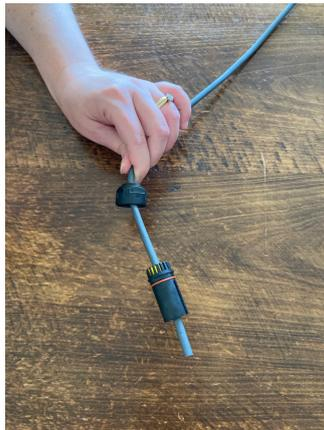
4. Strip the Starlink cable sheath back 25 mm from the end.
