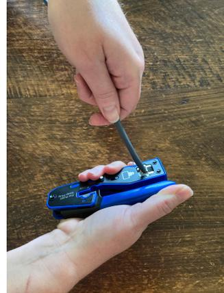
12. Remove the cable from the tool and check that all of the pins are down. If any of the pins aren't pushed down, put the wire back into the crimping tool and crimp it again.
