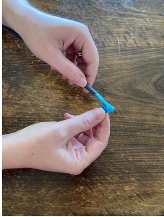
6. Fold the grounding wire back and remove the clear foil back to the cable sheath.
