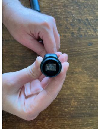
15. Push the insert into the Weatherproof plug and secure the cap back on the Weatherproof plug. The insert has a groove that is required to line up on the inside on the plug.
