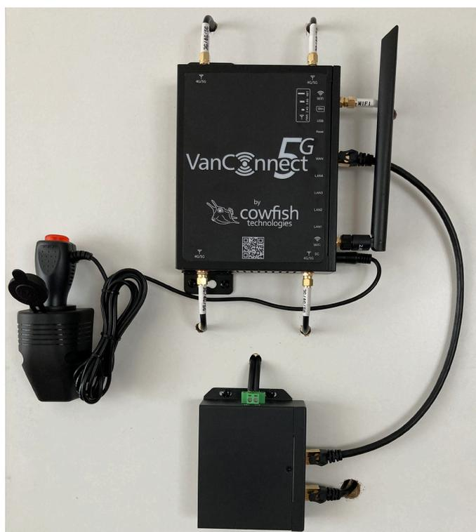
In order to supply input power to the 12V Dishy Power Supply, a minimum of 14 AWG electrical wire is required. This cable is to be connected to the 12V power source and correctly fused. Installation by a certified auto electrician is advised. The 12V Dishy Power Supply comes with a pluggable terminal block for easy wiring. Connect the 12V positive wire to the terminal labelled + and the 12V negative wire to the terminal labelled -
